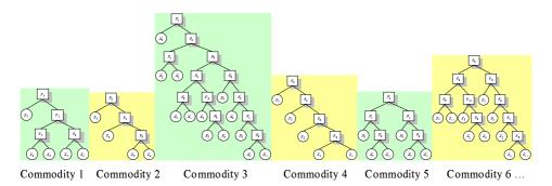
Fig. 1. A functional-modularity representation of commodities. Commodities are associated with their respective production processes which, when written in LIST programming language, can be depicted as parse trees as shown here.
